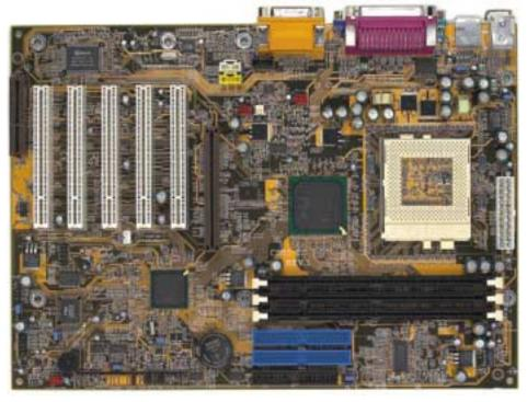
performance is needed. The CS65 provides 5 full-length PCI slots to support large system configurations. It also has a Communication and Networking Riser (CNR) slot for additional system flexibility. When the CNR slot is used, PCI expansion is four slots.
